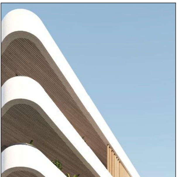
TC TIMBER-LOOK SOFFIT WOODFORM OR SIMILAR
